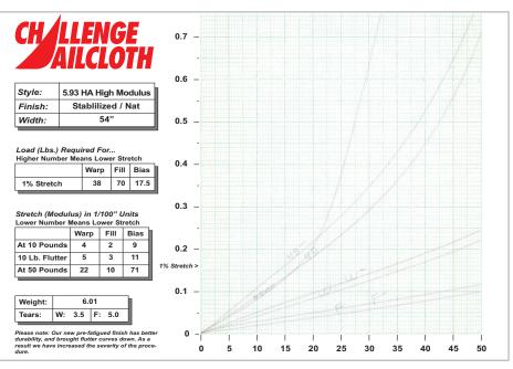
immersing the fabric in a bath of suspended resin. The resin is absorbed by the fiber. The cloth is fed into an oven where the liquids are driven off, leaving resin solids bonded to fibers. The fabric is heat-set several times, methodically shrunk at high termperature, further tightening the weave, and calendered at high tonnage to further stabilize the bias.
